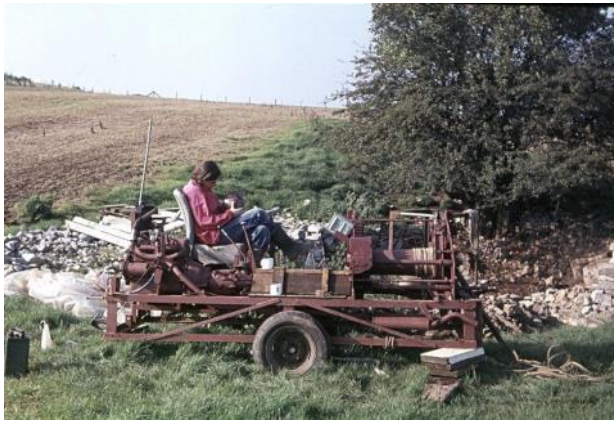
Photo 4. The old Stainsby's winch at Charterhouse Warren Farm Swallet modified with a Ford Anglia engine and mounted on a two wheeled angle-iron frame [Photo: T.Audsley, 1977?]
